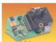
Connections: H=32 (including ports)  $+V_{\rm s}$  GND W = 30, D = 603 Fixing centres 52.4mm, 3.5mm dia.
